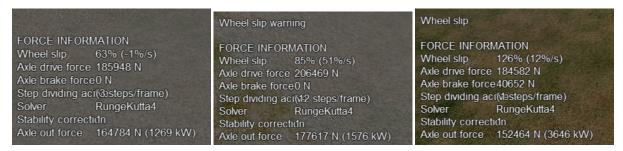
The actual maximum of the tractive force is based on the Curtius-Kniffler adhesion theory and can be adjusted by the aforementioned ORTSCurtius\_Kniffler ( A B C D ) parameters, where A, B, C are coefficients of Curtius-Kniffler, Kother or similar formula. By default, Curtius-Kniffler is used.
