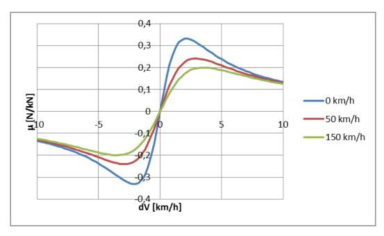
The wheel creep describes the stable area of the characteristics and is used in the most of the operation time. When the tractive force reaches the actual maximum of the slip characteristics, force transition falls down and more power is used to speed up the wheels, so called wheel slip.
