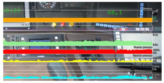
At the bottom of the picture, some moving graphs are displayed that show the actual load of the computer. Referring to memory use, about at least 400 MB must remain free to avoid out-of-memory exceptions
