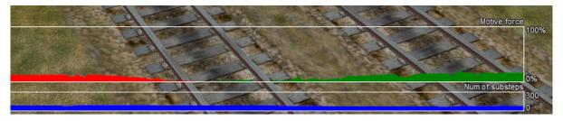
The upper graph displays the motive force in % of the player locomotive. Green colour means tractive force, red colour means dynamic brake force.
