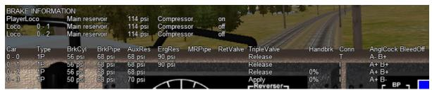
All of the hoses are now connected; only the angle cocks on the lead locomotive and the last car are closed as indicated by the -. The rest of the cocks are open (+) and the air hoses are joined together (all I) to connect to the air supply on the lead locomotive.
