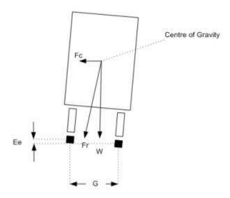
Fig. 2: Forces on rolling stock transitioning a curve
