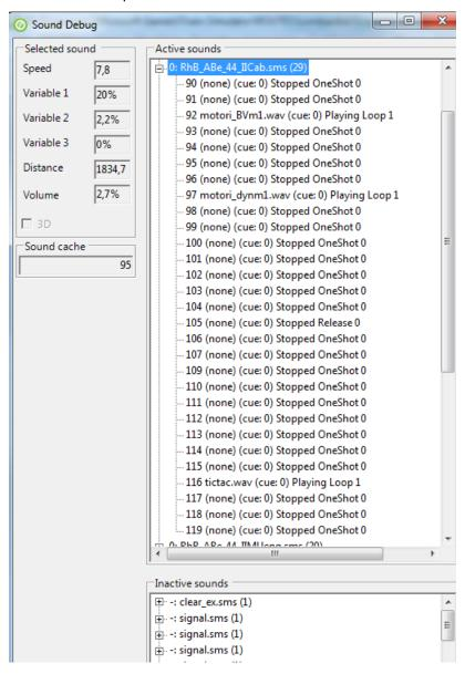
It shows in the upper part the list of all active .sms files (track sound apart); by expanding the detail of a specific .sms file, the list of all sound streams is displayed, as well as their state. On the left the value of the analog sound variables is displayed for the selected .sms file. The volume refers to the first stream of the selected sound file.
