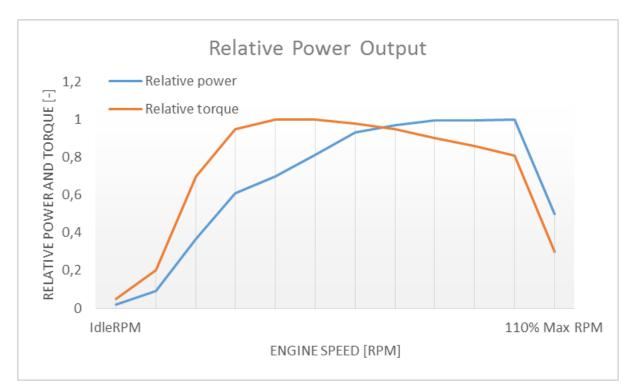
In many cases the throttle vs. speed curve is customized because power vs. speed is not linear. A default linear throttle vs. speed characteristics is built in to avoid engine overloading at lower throttle settings. Nevertheless, it is recommended to adjust the table below to get more realistic behavior.
