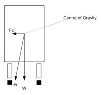
Fig. 4: Forces at work when a train rounds a curve
